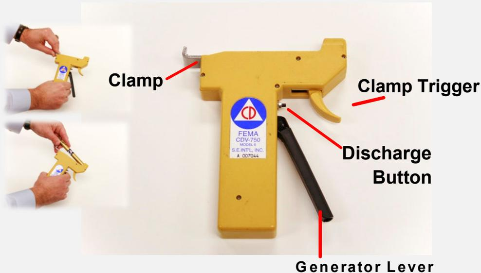
The dosimeter charger is used to charge or zero the pocket dosimeters with different lengths and ranges. The charger provides 200 volts to the direct-read dosimeter that moves the hairline down to zero.
