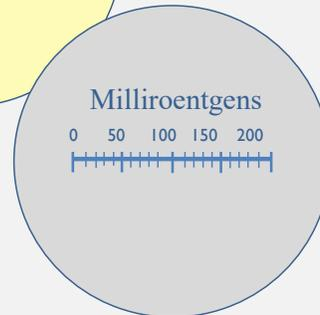
The Direct-Read Dosimeters (DRD) are designed to measure gamma radiation and x-rays. The DRD is a pencil-shaped tube with an eyepiece at the clip end and an ion-chamber equipped with a charging pin at the opposite end. Dosimeters are fairly accurate, rugged, and can be read directly by the user. Direct-Read Dosimeters give the advantage of immediately knowing the amount of gamma radiation that the wearer has been exposed to. DRDs are not expensive and are fairly easy to use.
